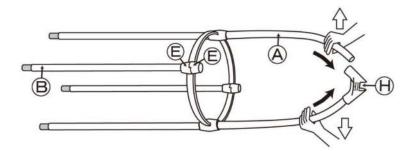
5. Continue connecting the 2 bends (A) with the whole structure, secured by connector 1 (G) and the connector 2 (H) and push them together.
