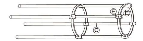
3. Slide the four long pipes (B) into the half ring (E), attach the 2 bends (A).
